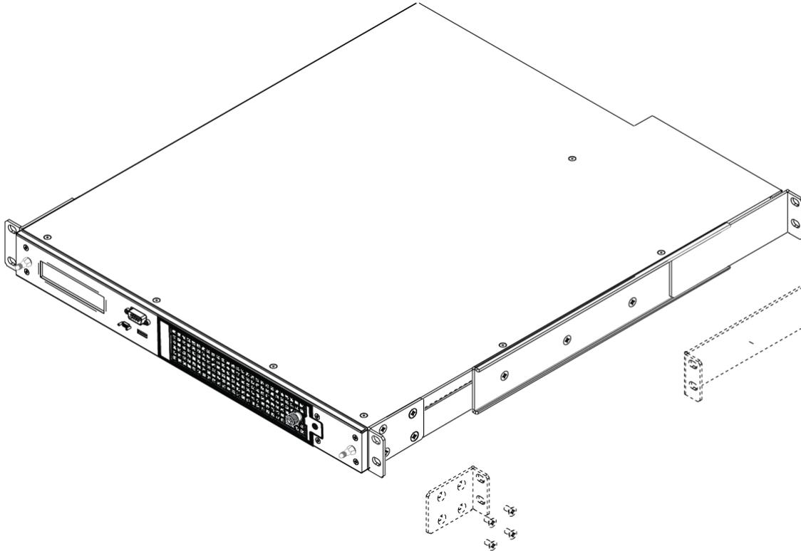
2. Mount the appliance in your equipment rack. Alternatively, ignore the rails and mounting tabs, and rest the Luna SA appliance on a mounting tray or shelf suitable for your specific style and brand of equipment rack.
