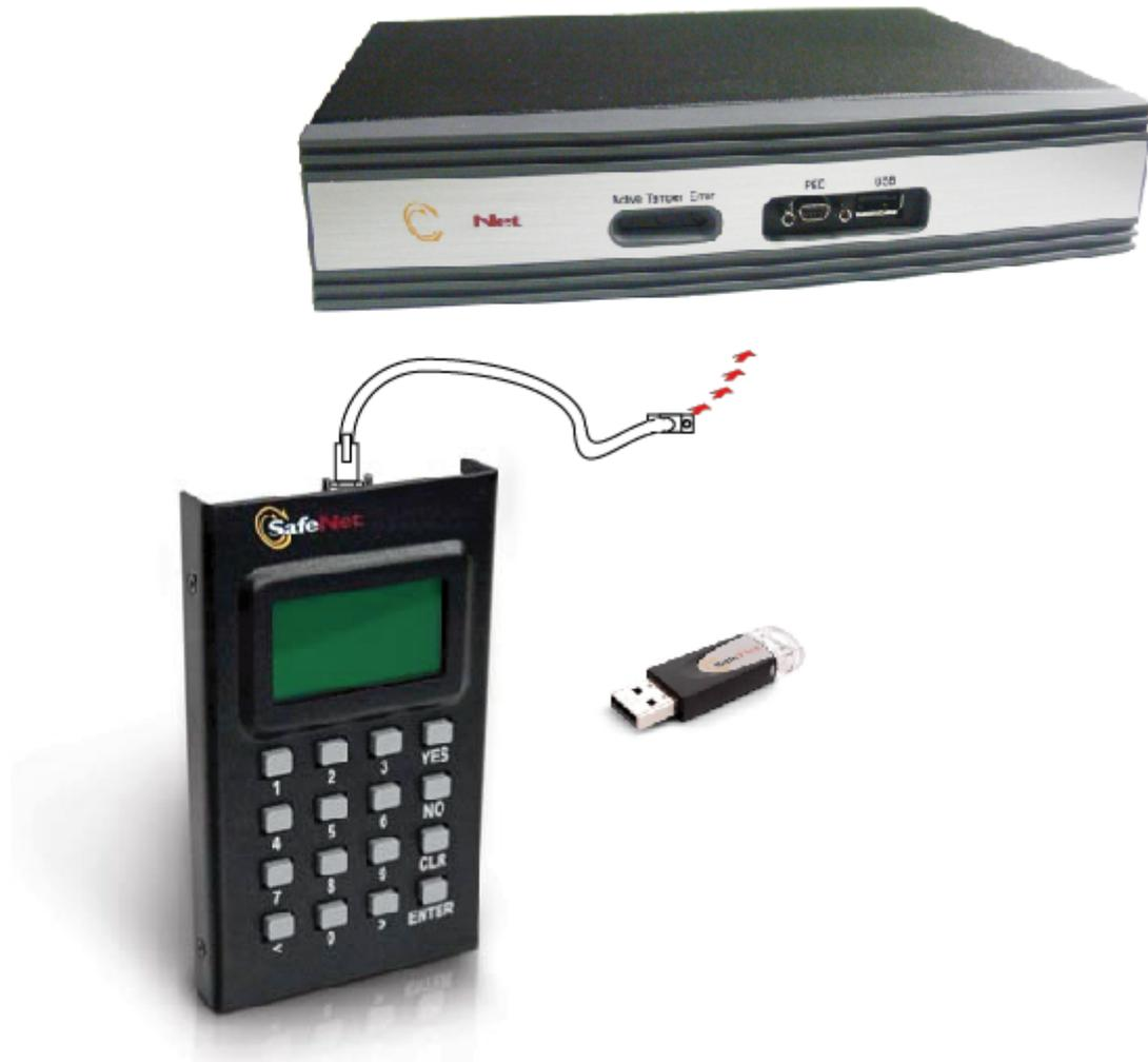
5. Using the USB cable, connect the Luna G5 to a USB port on the Luna client computer.
