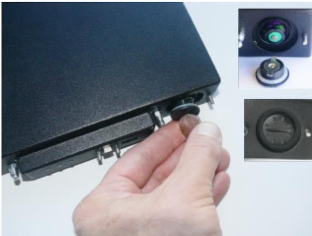
3. Remove the battery from its packaging and align it at the opening of the Luna G5 battery compartment. The battery should have a "+" sign near the end with the raised nub/bump. The flat end of the battery is the negative pole (-).
